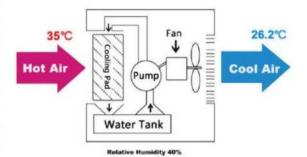
Portable evaporative air coolers are perfect natural cooling way to make freshing air to cool your body, compared to traditional air conditioning system, there are some benefits:
